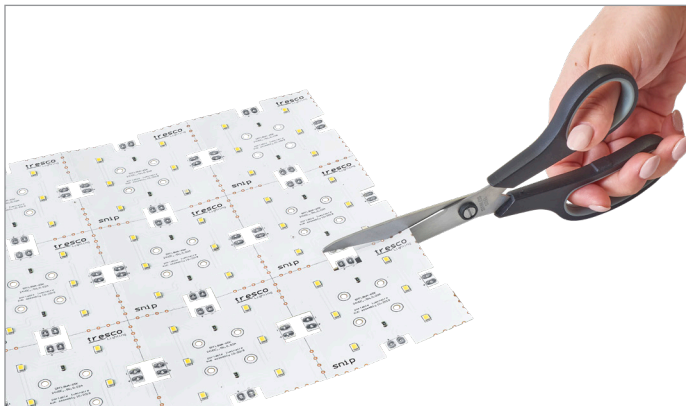
Cuttable and linkable modular DIY lighting system
